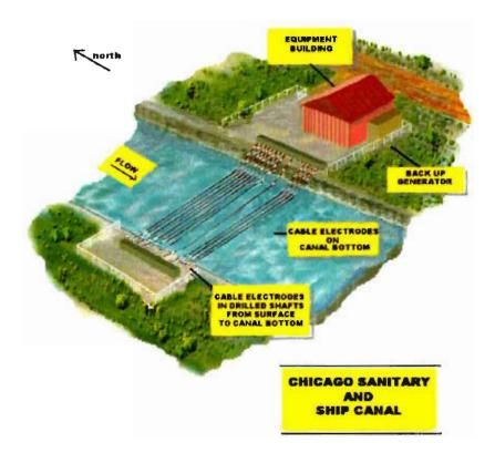
Figure 2: Plan view of how barrier electrodes are placed in canal bottom. (Source: http://images.suite101static.com/792724\_com\_db1.jpg (last accessed, October 7, 2010)
