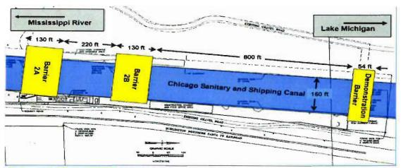
Figure 3: Illustration of the Chicago Sanitary and Ship Canal Aquatic Nuisance Species Dispersal Barriers in Romeoville, IL.
